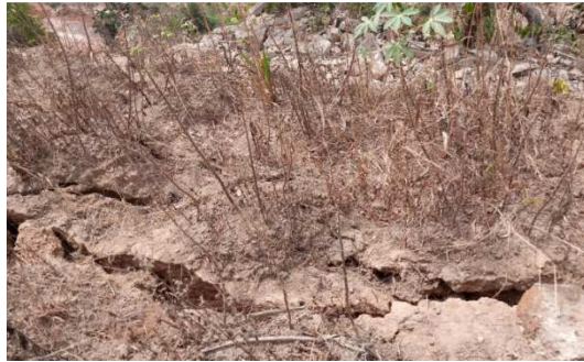
Figure 3. Cracks on the land adjacent to the landslide.
